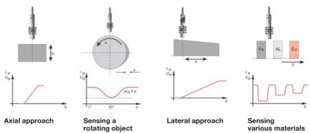
Distance changes in the sensor axis result in proportionally changing output signals.
